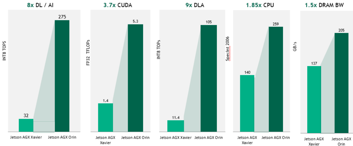
Figure: 1 Jetson AGX Orin delivers 8X the AI performance of Jetson AGX Xavier
