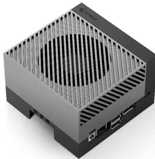
Figure 13: Jetson AGX Orin Developer Kit
